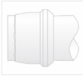
Fig. T47 — Tube not bottomed
