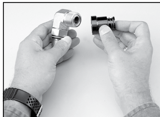
Fig. S25 – O-Ring installation using the CORG assembly tool
