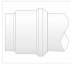
Fig. T48 — Shallow bite
